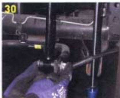
THE SWAY BAR IS HOOKED UP WITH EXTENDED LINKS.
