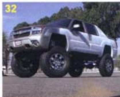
HERE IS THE TRUCK WITH ALL ITS ADDED LIFT. THE CST SUSPENSION WORKS FLAWLESSLY AND HAS A NICE ON-ROAD MANNERISM, BUT IT STILL HAS OFF-ROAD PROWESS. SOCAL SUPERTRUCKS RECOMMENDS THAT WHENEVER YOU LIFT YOUR TRUCK, RETURN TO THE SHOP AFTER A WEEK OR SO TO HAVE THE BOLTS RETORQUED BECAUSE THE SUB FRAMES WILL SET.
