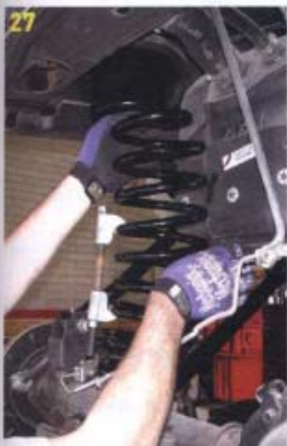
NOW THE 4-INCH LIFT COIL IS INSTALLED.
