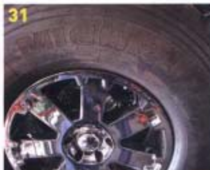
THE WHEELS AND TIRES USED ON THIS TRUCK ARE ALSO 20X30-INCH KMC ZIPPER. THEY FEATURE A CHROME FINISH AND ARE LOAD RATED TO HANDLE THE ADDED WEIGHT OF THE MASSIVE 11.00X23-INCH MICHELIN XZLS, WHICH MEASURE 42 INCHES O.D.
