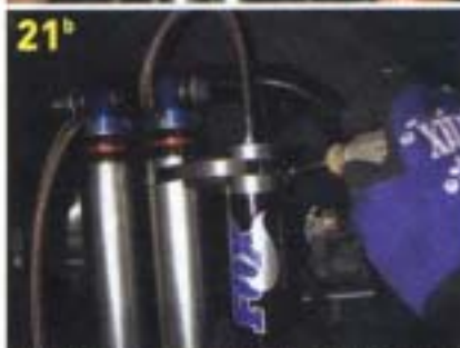
21 THE SHOCKS WERE NEXT. AFTER THE HOOP WAS BOLTED IN, THE DUAL FOX SHOCKS SLIPPED RIGHT INTO PLACE.
