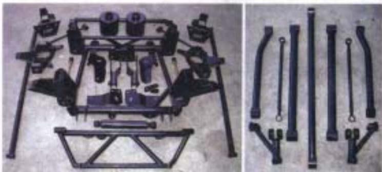
HERE ARE ALL THE CST LIFT COMPONENTS THAT WILL RAISE THE TRUCK A TOTAL OF 12 INCHES. THE KIT IS CONSTRUCTED OF DOM (DRAWN OVER MANDREL) TUBING AND 1/4-INCH PLATE STEEL. ALL JOINTS ARE TIG-WELDED, AND THE ENTIRE KIT IS POWDERCOATED GLOSS BLACK. WHAT MAKES THIS KIT DIFFERENT THEN THE REST IS THAT THE FRONT DROP DOWN BRACKETS HAVE BEEN MADE INTO A SINGLE SUB FRAME.
