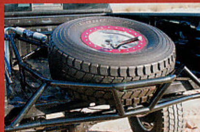
▲ CST fabricated the clean and simple bedcage for the Titan, making room for a spare 37x12.50R17 BFGoodrich Project Baja T/A tire and KMC wheel.
