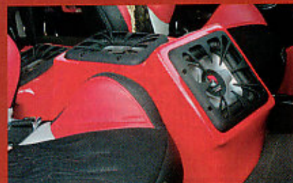
center console houses three Kicker Solobaric LT square subwoofers, while the custom-painted amp rack keeps the amps from flying around during hard hits. A Sony head unit takes charge of the system and Kicker component speakers reproduce the mid-bass and high frequencies.
