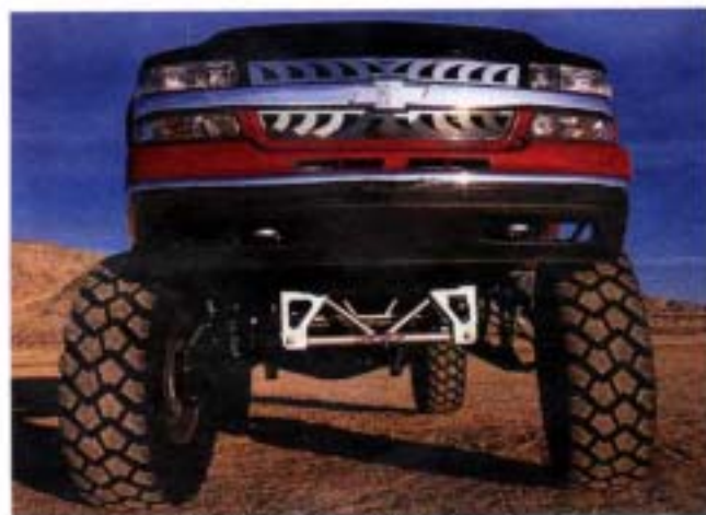
▲ John designed and fabricated the beautiful wishbone upper link and the lower ladder bars. The wishbone pivots on chromoly rod ends while the ladder bars swing on Delrin bushings.
