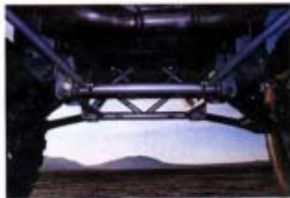
▲ The majority of front-end lift can be credited to the CST 9-inch drop-down cradle. This beauty lays both the upper and lower control arms well beneath the fenderails, and the strut bars keep the cradle held firmly in place.
