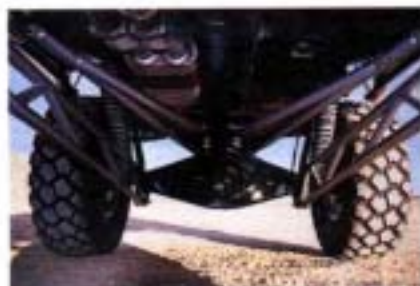
▲ John designed and fabricated the beautiful wishbone upper link and the lower ladder bars. The wishbone pivots on chromoly rod ends while the ladder bars swing on Delrin bushings.
